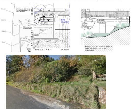
From Endeavour Energy's perspective the fact that provision is being made for a padmount substation is a positive (which may facilitate the removal of pole mounted substation no. 9360). Endeavour Energy's general requirements is for a padmount substation to be at ground level and have direct access from a public street (unless provided with appropriate easements for the associated underground cables and right of access).
